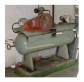
Compressors should be mounted preferrably in an outside enclosure because it is a pressurised unit.
